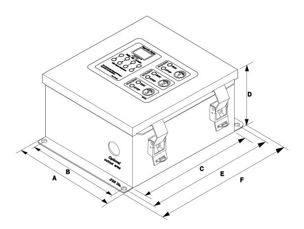
The DIN-rail Controller can be either DIN-rail mounted or screwed down. Be sure to allow space for wiring to top of box (both sides).
