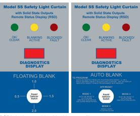
The (RSD) device provides blanking scrolling operator diagnostic message display and system status <u>without</u> entry into the machine control panel. This saves time for lockout/tagout requirements and safeguarding blanking adjustments.
