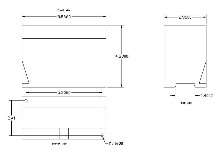
**Enclosure:** Gray polycarbonate with clear cover. Provides IP40, UL94V-1
