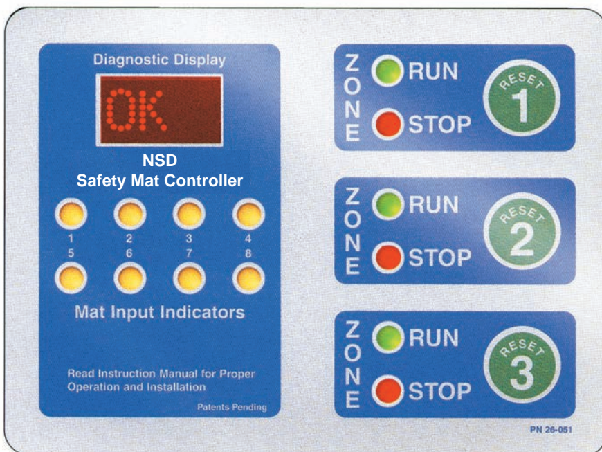
Controller Display front panel with diagnostic display and multiple zone resets
